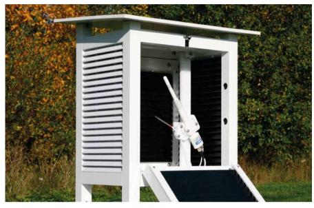
*HMP155 with an additional temperature probe and optional Stevenson screen installation kit.*
