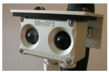
The sensor is sensitive for particles in a zone about 25 cm ahead of the location of the sensor that limit the visibility in the air. These particles are normally the microscopic water particles constituting fog, but they may also be snowflakes, raindrops or air pollutants. But the particle density must be high enough to limit the visibility to lower than about 2000 meters. The sensor is heated to a few degrees above ambient temperature in order to keep moisture away
